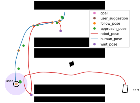
Fig. 9. Results from a user following test, where the cart was asked to follow the user at a distance of R_{f \rightarrow w} = 1 m. The cart initially follows the user until it reaches R_{f \rightarrow w} , and then moves to the suggested waiting pose (purple). The robot resumes following once the user moves further than R_{w \rightarrow f} .
